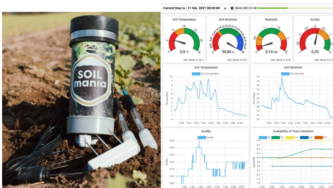
Figure 10: TreeMania soil health sensors (left) and snippet of the dashboard (right). Source: TreeMania
